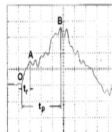
Figure 3. A typical VFTO waveform. Time Scale: 2.5 ns/div. t_r = Breakdown time. t_p = time to maximum peak. O: is at 10% of the peak value (B) obtained with zero (0 V) as the base. A: is the first peak from O on the rising portion of the VFTO waveform. B: maximum peak of the VFTO
